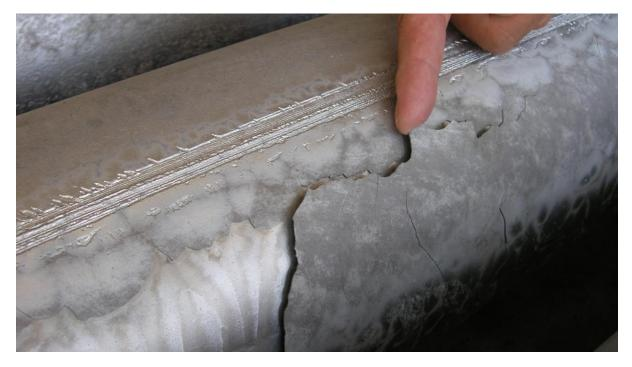
**Figure 3:** The zinc coaing is flaking off a fabricated pipe due to the steel chemistry. The mottled grey appearance is indicative of a silicon content between 0.04% and 0.14% (see *TN Mottled Appearance*).
