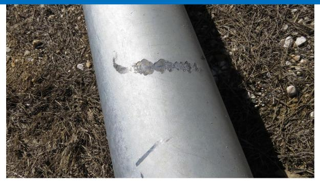
Figure 7: Impact during handling has caused flaking of the thick, brittle galvanized coating.
