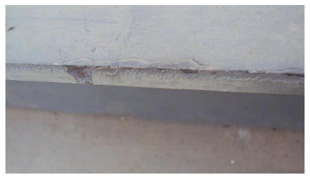
Figure 6: Handling damage has caused flaking near the edge of the galvanized article.
