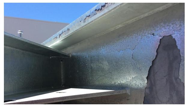
**Figure 1:** The galvanized coating is flaking off on multiple places of the article. Depending on the size of the bare spots and end use it may need to be regalvanized.
