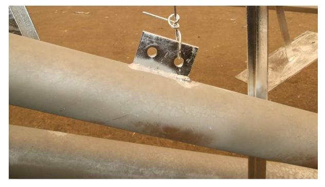
**Figure 2:** The majority of the pipe has a matte grey appearance, most likely due to the steel chemistry.
