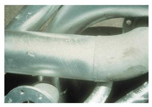
**Figure 7:** The shiny surface (to the left) is typical of Category X, A & B, while the duller coating (to the right) is typical of Category C & D. Over time, the both coatings will weather and tend towards a similar dull grey colour. This product meets the requirements of AS/NZS 4680.
