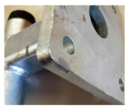
**Figure 5:** Handling has caused some damage to the edge of this thick galvanized coating, where some of the coating has been chipped. Thick coatings can result when steels from Categories C & D are galvanized. It is likely the coating will still meet the thickness requirements of AS/NZS 4680, and is acceptable, so long as the remaining product firmly adheres to the substrate.
