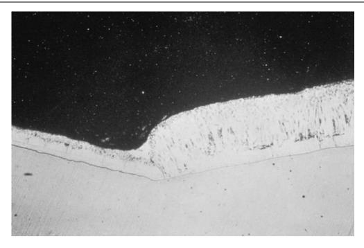
**Figure 8:** The join between the shiny and dull coatings of Figure 7 showing the thinner coating achieved in Category X, A & B on the left compared to the thicker and more brittle coating achieved with Category C & D to the right.
