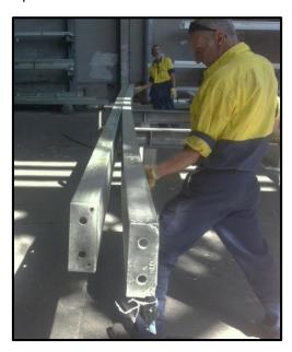
Two identical fabricated PFC sections galvanized at the same time with vastly different deformation
