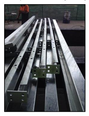
Fabricated PFC sections with a shallow curve along the welded face
