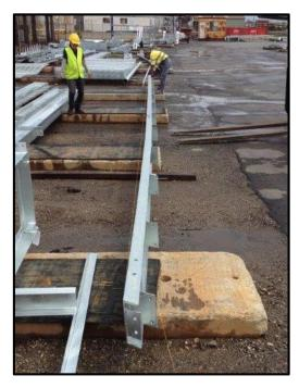
A fabricated PFC that has distorted during the galvanizing process
